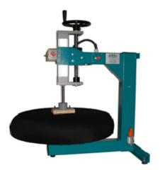
With special turnable foam cushion to upholstery a big range of different models of chair seats and backrests. For safety the press is working with two hand sensor control device. Pressure regulator and main air switcher is included.
